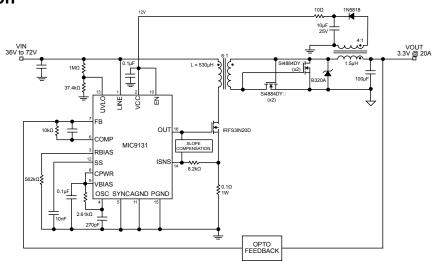
90% Efficient Telecommunications Power Supply
