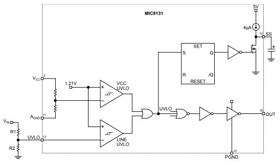
Figure 4: UVLO and Soft Start Circuits
