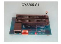
To accommodate the largest number of pin counts with each board, the largest socket is installed. For example, the CY3205-S1 includes a 48-pin DIP socket. It therefore supports 8, 20, 28, and 48-pin DIP parts. The CY3205-S3 includes a 28-pin SSOP socket that can accept both the 20 and 28-pin SSOP parts. The body width of the 48-pin SSOP package is wider than the 20 and 28-pin so the CY3205-S4 is necessary for the 48-pin SSOP parts.
