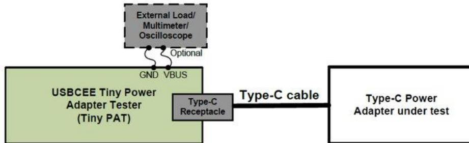
*USBCEE Tiny PAT System Setup*
