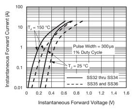
Fig. 3 - Typical Instantaneous Forward Characteristics
