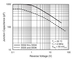
Fig. 5 - Typical Junction Capacitance
