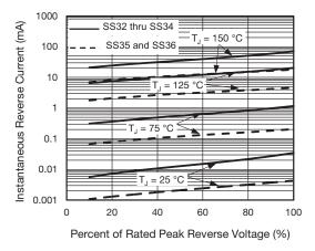
Fig. 4 - Typical Reverse Current Characteristics
