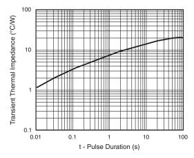
Fig. 6 - Typical Transient Thermal Impedance
