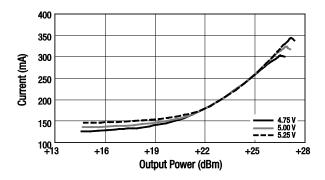
Figure 64. Operational Current vs Output Power Over Voltage
