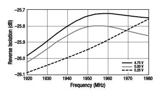
Figure 48. Reverse Isolation vs Frequency Over Voltage
