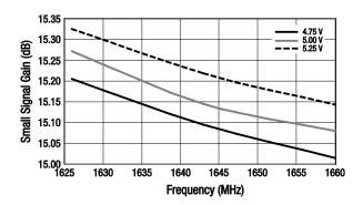
Figure 3. Small Signal Gain vs Frequency Over Voltage
