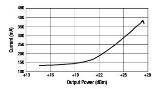
Figure 22. Operational Current vs Output Power
