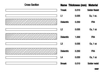
**Figure 69. Layer Detail Physical Characteristics**
