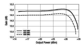
Figure 50. Gain vs Output Power Over Frequency
