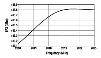
Figure 62. IIP3 vs Frequency (PIN = -10 dBm)
