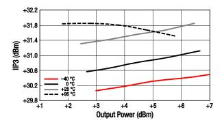
Figure 37. IIP3 vs Output Power Over Temperature
