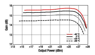
Figure 33. Gain vs Output Power Over Temperature
