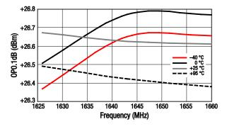
Figure 13. OPO.1dB vs Frequency Over Temperature
