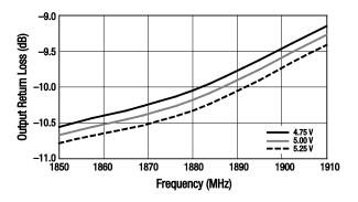
Figure 28. Output Return Loss vs Frequency Over Voltage
