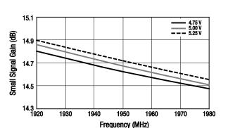
Figure 47. Small Signal Gain vs Frequency Over Voltage
