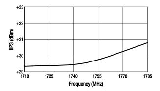
Figure 20. IIP3 vs Frequency (PIN = -10 dBm)
