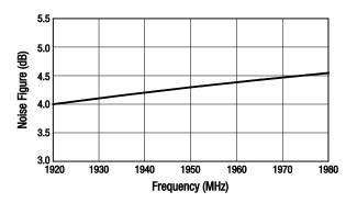
Figure 54. Noise Figure vs Frequency
