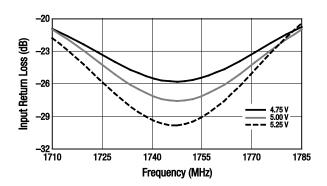
Figure 14. Input Return Loss vs Frequency Over Voltage
