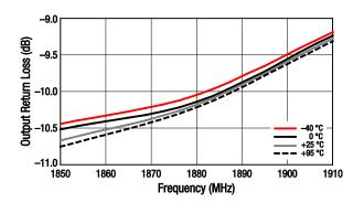
Figure 27. Output Return Loss vs Frequency Over Temperature
