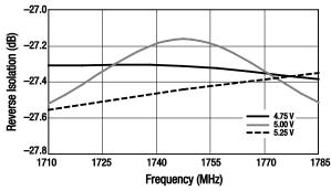
Figure 17. Reverse Isolation vs Frequency Over Voltage
