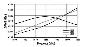
Figure 36. OP1dB vs Frequency Over Voltage
