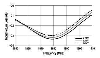
Figure 26. Input Return Loss vs Frequency Over Voltage
