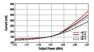
Figure 41. Operational Current vs Output Power Over Temperature
