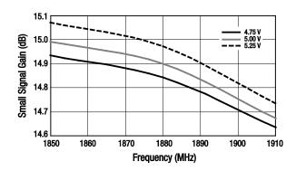
Figure 30. Small Signal Gain vs Frequency Over Voltage
