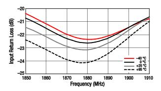
Figure 25. Input Return Loss vs Frequency Over Temperature
