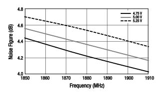
**Figure 40. Noise Figure vs Frequency Over Voltage**
