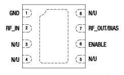
Figure 2. SKY65095-360LF Pinout – 8-Pin DFN Package (Top View)
