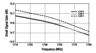
Figure 16. Small Signal Gain vs Frequency Over Voltage
