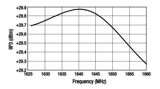
Figure 10. IIP3 vs Frequency (PiN = -10 dBm)
