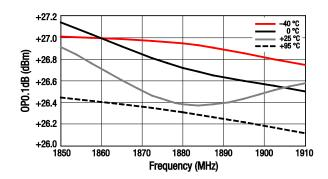
Figure 44. OPO.1dB vs Frequency Over Temperature
