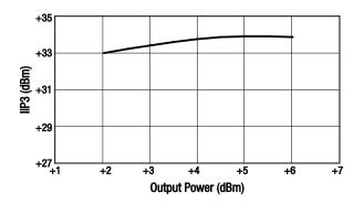
Figure 63. IIP3 vs Output Power
