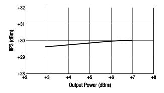
Figure 9. IIP3 vs Output Power
