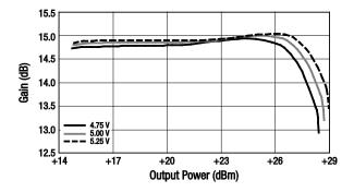
Figure 49. Gain vs Output Power Over Voltage
