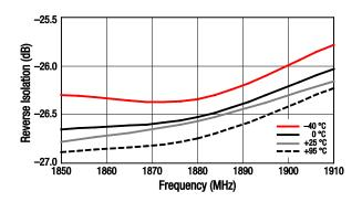
Figure 31. Reverse Isolation vs Frequency Over Temperature
