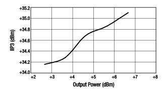
Figure 52. IIP3 vs Output Power
