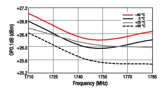
Figure 24. OP0.1dB vs Frequency Over Temperature
