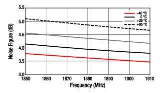
Figure 39. Noise Figure vs Frequency Over Temperature
