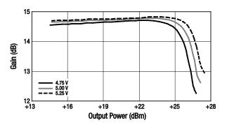
Figure 61. Gain vs Output Power Over Voltage
