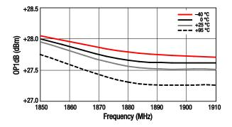
Figure 35. OP1dB vs Frequency Over Temperature
