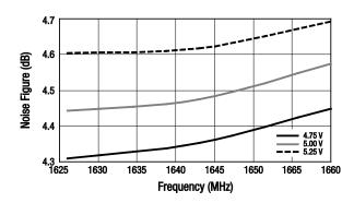
Figure 12. Noise Figure vs Frequency Over Voltage
