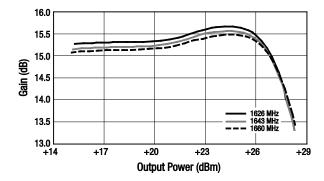
Figure 8. Gain vs Output Power Over Frequency
