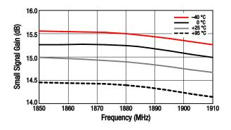
Figure 29. Small Signal Gain vs Frequency Over Temperature
