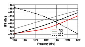
Figure 38. IIP3 vs Frequency Over Temperature
