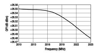
Figure 60. OP1dB vs Frequency
