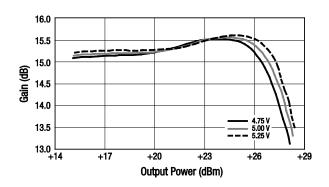
Figure 7. Gain vs Output Power Over Voltage
