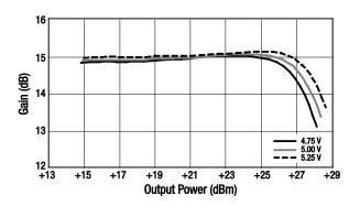
Figure 34. Gain vs Output Power Over Voltage
