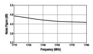
Figure 23. Noise Figure vs Frequency
