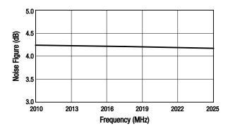
Figure 65. Noise Figure vs Frequency
