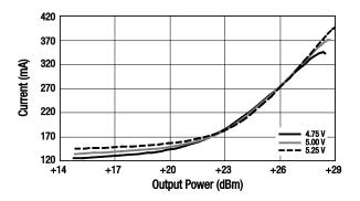
Figure 53. Operational Current vs Output Power Over Voltage
