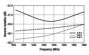
**Figure 6. Reverse Isolation vs Frequency Over Voltage**
