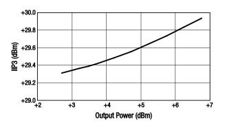
Figure 21. IIP3 vs Output Power
