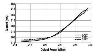
Figure 11. Operational Current vs Output Power Over Voltage
