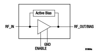
Figure 1. SKY65095-360LF Functional Block Diagram
