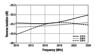
Figure 59. Reverse Isolation vs Frequency Over Voltage
