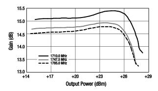
Figure 19. Gain vs Output Power Over Frequency
