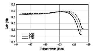
Figure 18. Gaim vs Output Power Over Voltage
