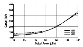
Figure 42. Operational Current vs Output Power Over Voltage
