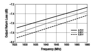
Figure 5. Output Return Loss vs Frequency Over Voltage
