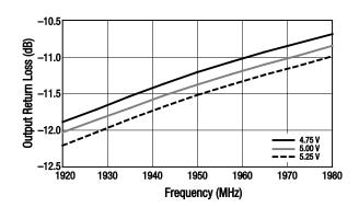
Figure 46. Output Return Loss vs Frequency Over Voltage
