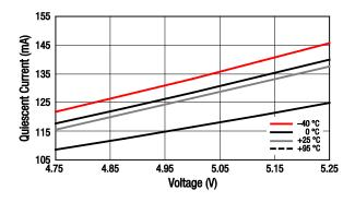
Figure 43. Quiescent Current vs Voltage Over Temperature
