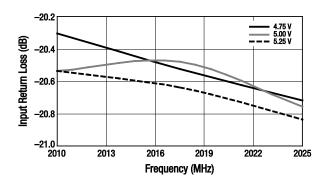
Figure 56. Input Return Loss vs Frequency Over Voltage
