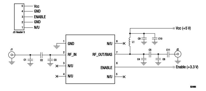
Figure 70. SKY65095-360LF Evaluation Board Schematic
