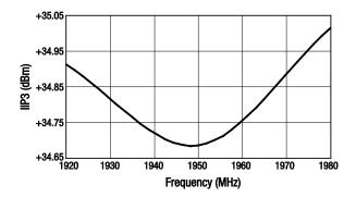
Figure 51. IIP3 vs Frequency (PIN = -10 dBm)
