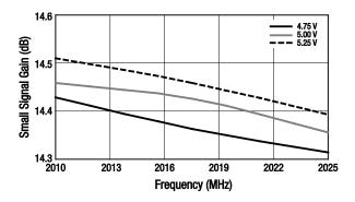
Figure 58. Small Signal Gain vs Frequency Over Voltage
