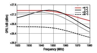
Figure 55. OP0.1dB vs Frequency Over Temperature
