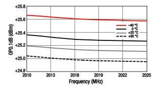
Figure 66. OPO.1dB vs Frequency Over Temperature
