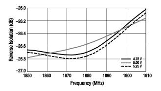
Figure 32. Reverse Isolation vs Frequency Over Voltage
