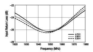
Figure 45. Input Return Loss vs Frequency Over Voltage
