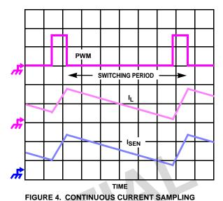
The ISL6323B supports Inductor DCR current sensing to continuously sample each channel's current for channel-current
