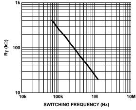
FIGURE 24. RT vs SWITCHING FREQUENCY
