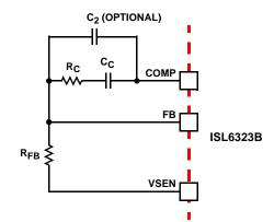
FIGURE 22. COMPENSATION CONFIGURATION FOR LOAD-LINE REGULATED ISL6323B CIRCUIT
