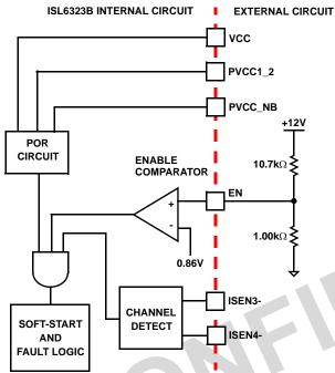
FIGURE 12. POWER SEQUENCING USING THRESHOLD-SENSITIVE ENABLE (EN) FUNCTION
