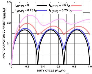
FIGURE 26. NORMALIZED INPUT-CAPACITOR RMS CURRENT FOR 3-PHASE CONVERTER
